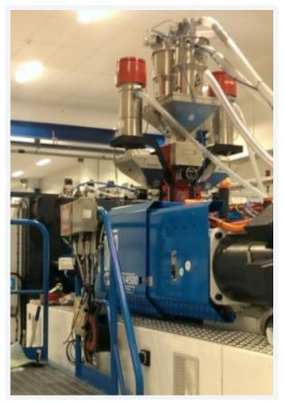
The MCHybrid blender is a unique dosing concept that combines two technologies into one system: batch blending and in-line dosing.
