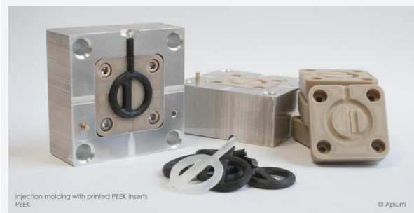
Figure 1: PEEK mold inserts with ABS (black) and Polyurethane (transparent) molded parts
