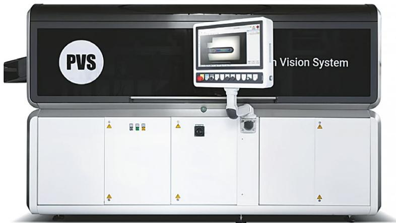
**W**ith the PVS10L, SACMI renews its mission to achieve total quality control of the product by using both in-line and stand-alone inspection solutions. More specifically, the PVS10L enhances the SACMI machine family for in-line and sample inspection by incorporating computer vision systems with new AI tools.
