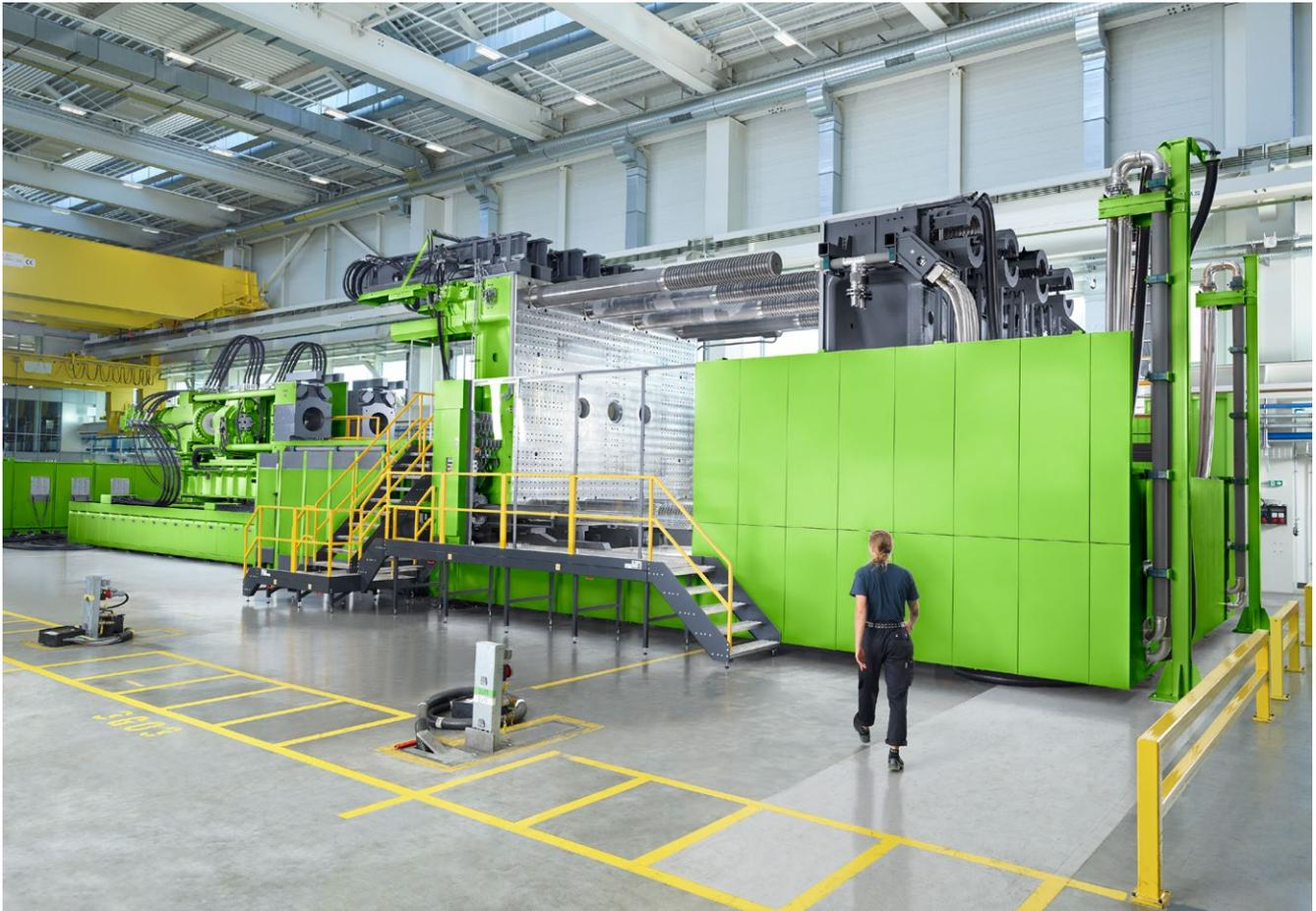
three ENGEL easix articulated robots for preparing large quantities of metal inserts and for handling the thermoplastic sheet, an ENGEL viper 90 linear robot and an ENGEL IR oven.
