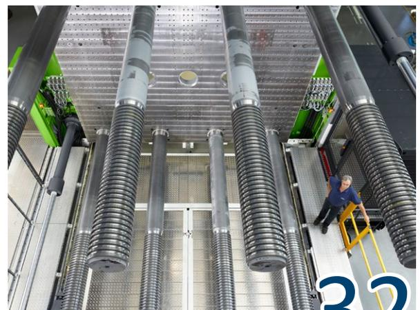
While ENGEL duo injection moulding machines have been available with clamping forces of up to 5500 tonnes as standard machines for a long time, ENGEL has now extended the series upwards for new applications in the mobility sector and other industries. Besides parts with a particularly large surface area and volume, these new mega machines with their extremely large mould mounting spaces enable even more extensive process integration – for example in the glazing sector.
